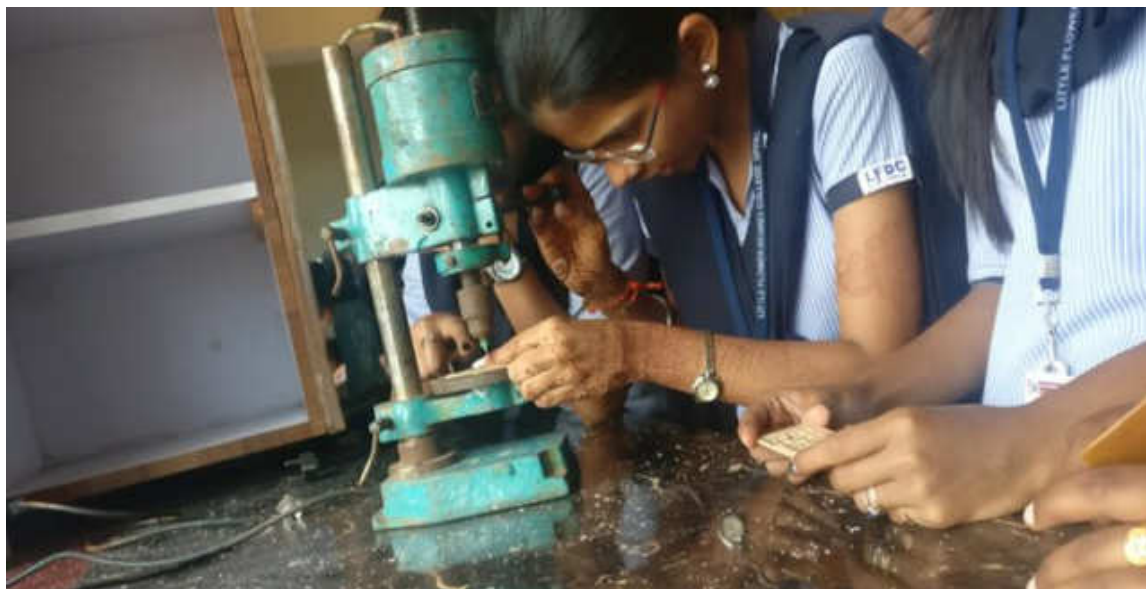
Students of B.SC MECS drilling holes in the PCB before connecting components
